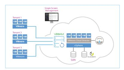
Deploy Veeam at the client site or at MSP site. Cloudian provides a shared, scalable backup target. VMware VCD enables single-screen management, end-to-end.
